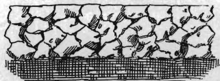
Stone on a macadam road, firmly wedged and packed together. Small stones, gravel, dirt or sand if mixed with the stone or spread at the surface before rolling, prevent its being thoroughly wedged and packed.
