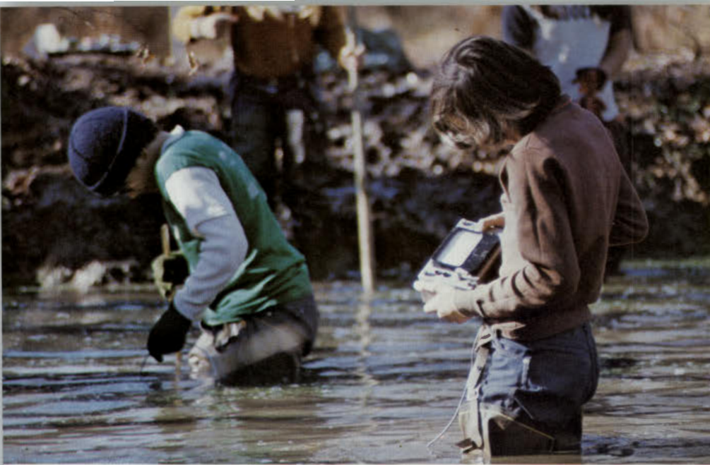
Pond-profile measurements are taken. Pond depths are obtained every few meters with a meter stick, while other students record water temperatures at the surface, middle, and bottom of pond.
