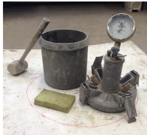
Figure 9. ASTM C231 Type B Pressure Air Meter
