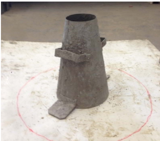
Figure 8. ASTM C134 Slump Test Setup
