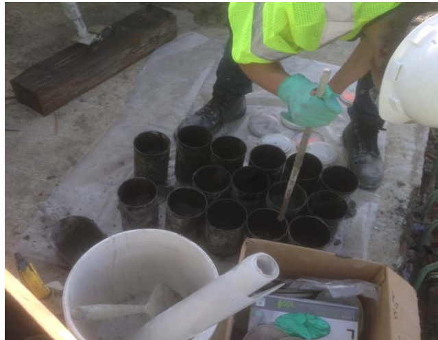
Figure 13. Rodding Fresh Concrete in Molds
