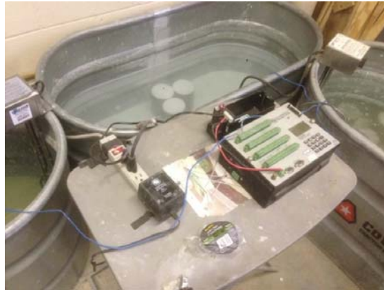
Figure 19 Accelerated (Hot) Lime Bath Curing
