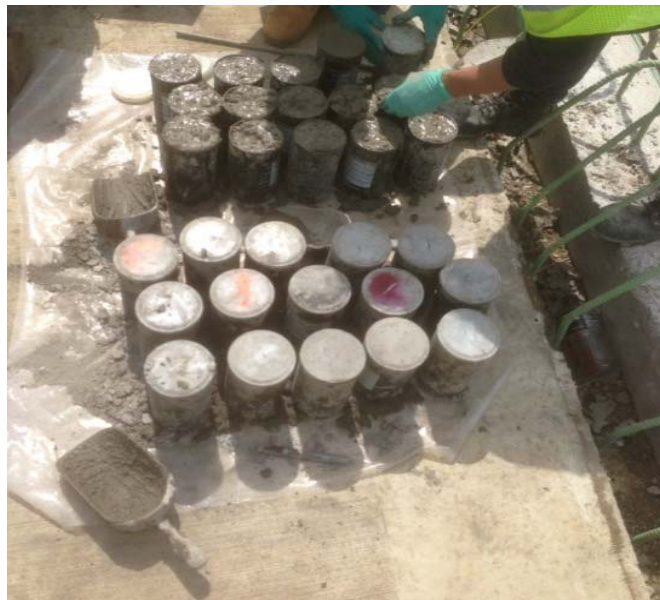
Figure 14. Covering Molds with lids to prevent evaporation
