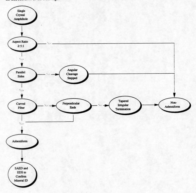
However, for some mineral particles, a more complex scheme (as shown in the next flowchart) is needed to determine asbestiform/cleavage. This second flowchart incorporates additional analyses particularly
