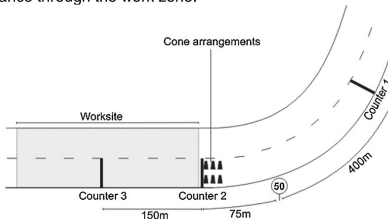
Figure 4. Worksite Layout (Allpress, 2010)<sup>(76)</sup>
