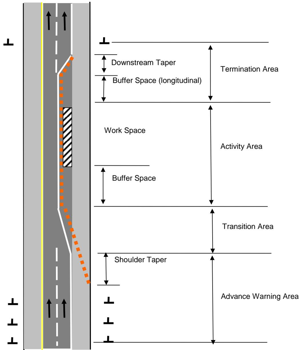
Figure 1. Component Parts of a Temporary Traffic Control Zone (MUTCD, 2009)<sup>(63)</sup>
