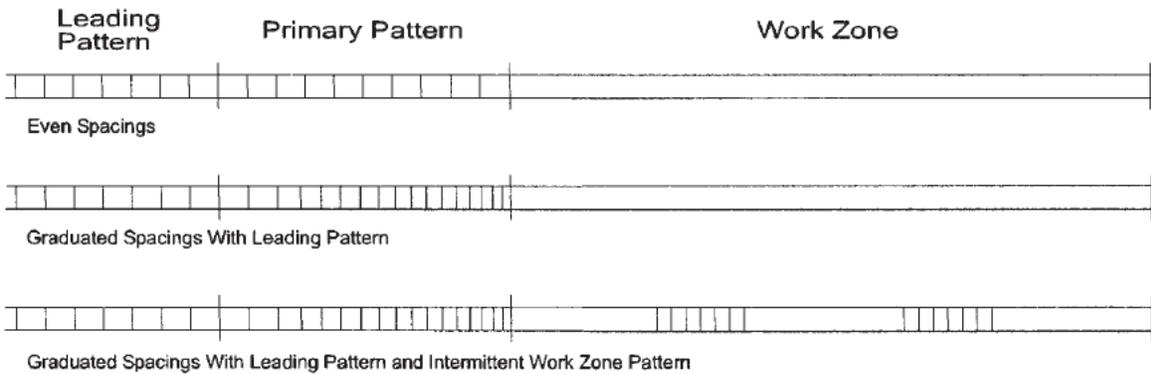
Figure 6. Optical Speed Bar Test Pattern (Meyer, 1999) <sup>(77)</sup>
