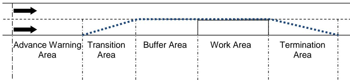
Figure 7. Component Segments of the Work Zone
