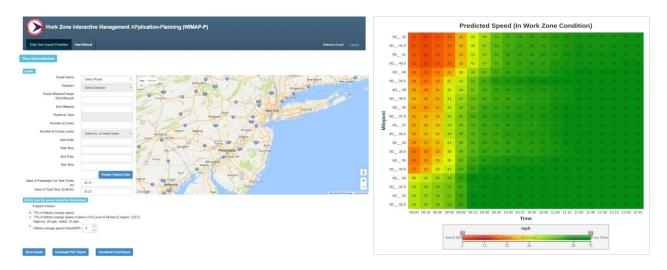
The Artificial Neural Network (ANN) and Multivariate Non-linear Regression (MNR) models were developed based on 466 work zones, which are employed by WIMAP-P to predict speed caused by work zones on NJ freeways and arterials. It was found that the ANN model is slightly more accurate for predicting delays of historic work zones, but the MNR model demonstrated better reliability and consistency in predicting delays of work zones in places where there are no historic data.
