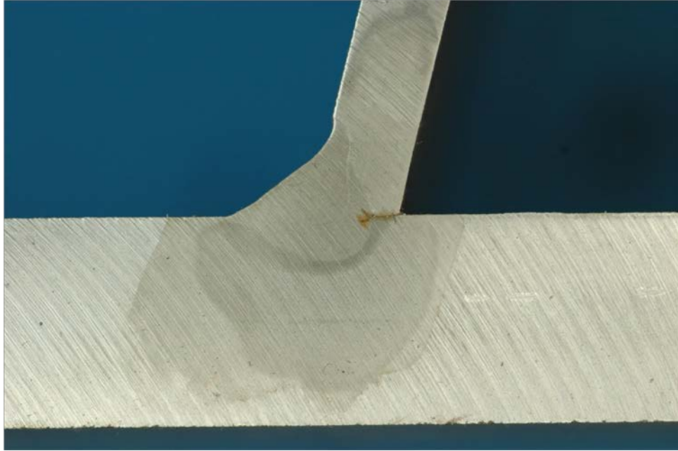
Figure 591. Macro-etched section R3_A_18
