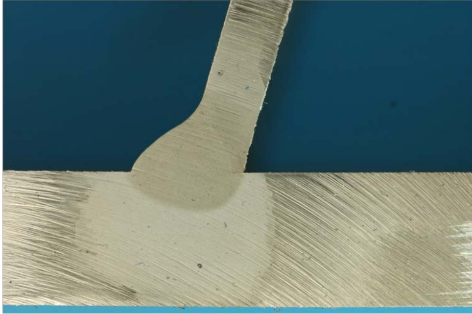
Figure 633. Macro-etched section A_84
