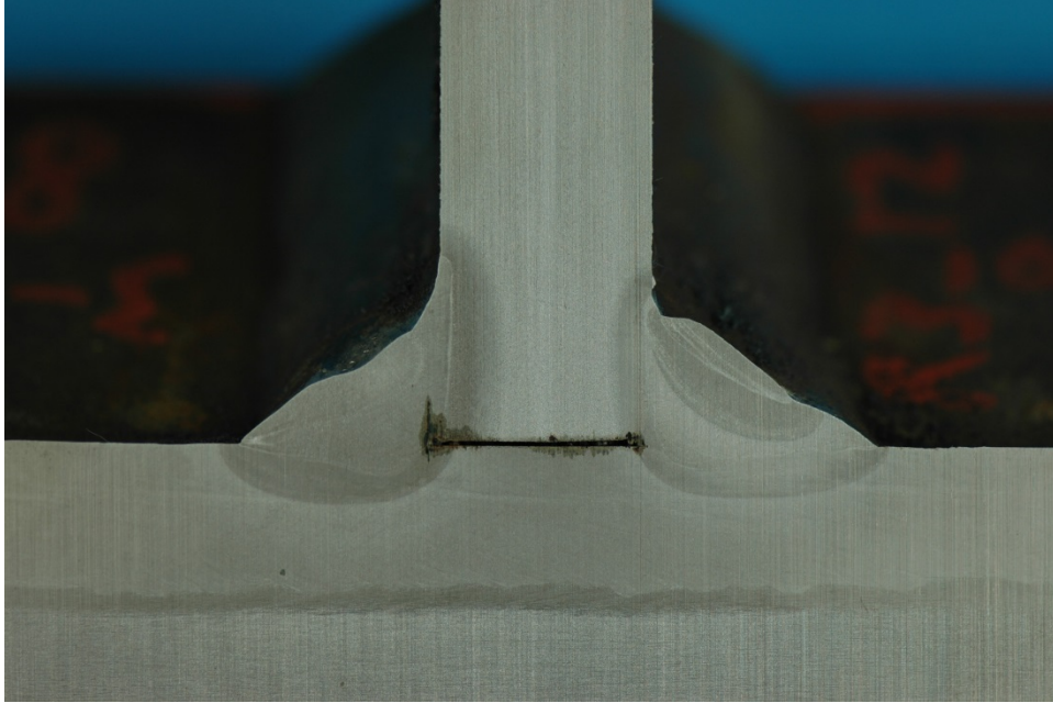
Figure 710. Macro-etched section R3_156_1
