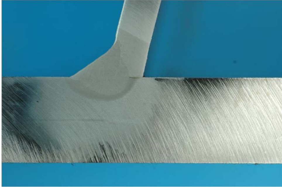
Figure 589. Macro-etched section R3_A_6
