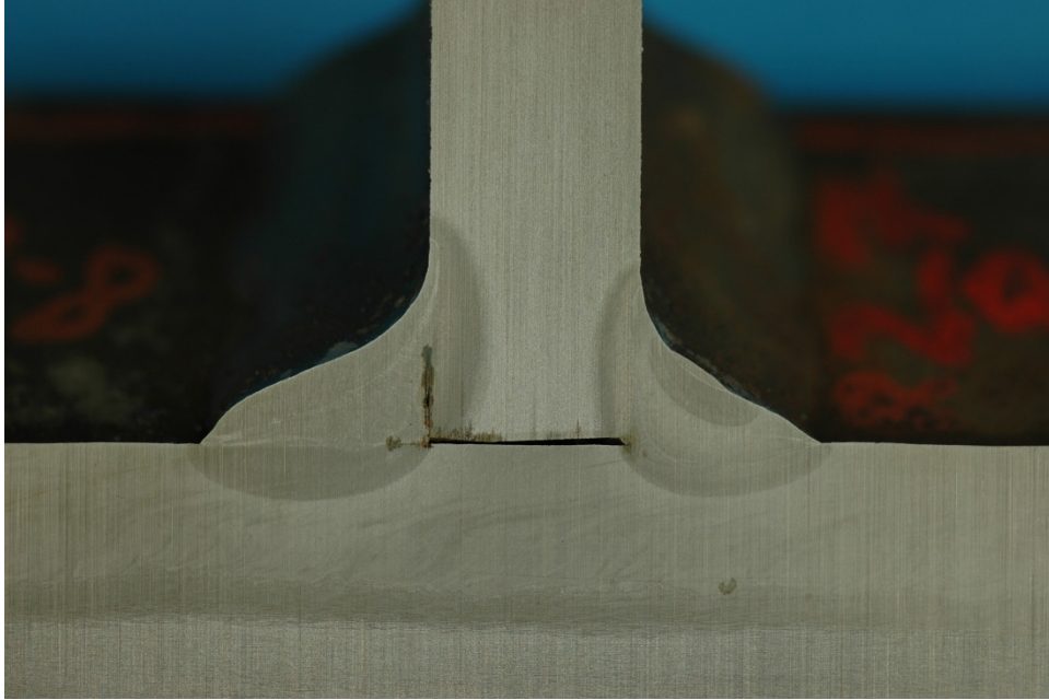
Figure 688. Macro-etched section R2_90_7
