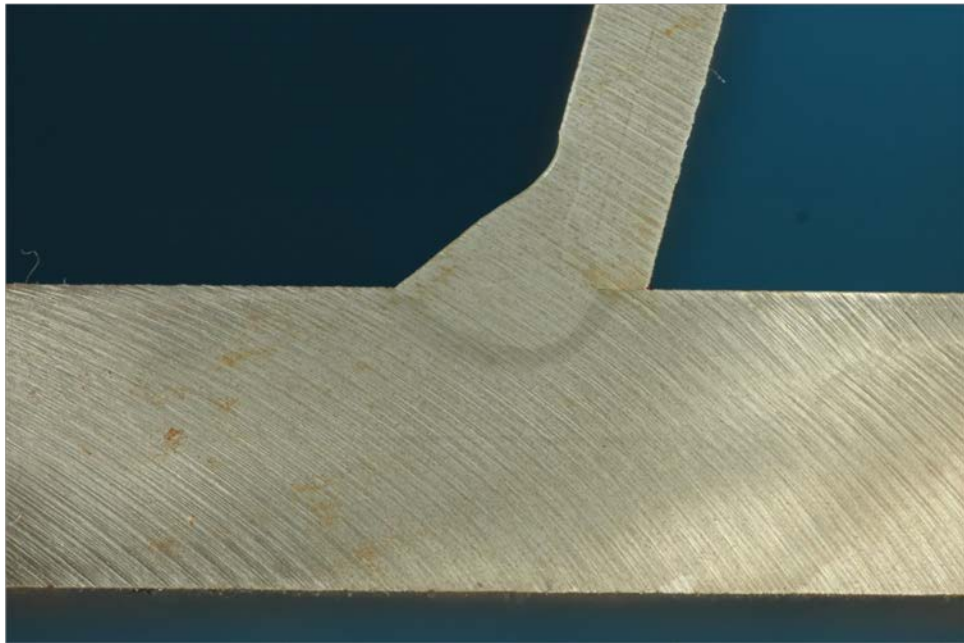
Figure 610. Macro-etched section R3_B_120
