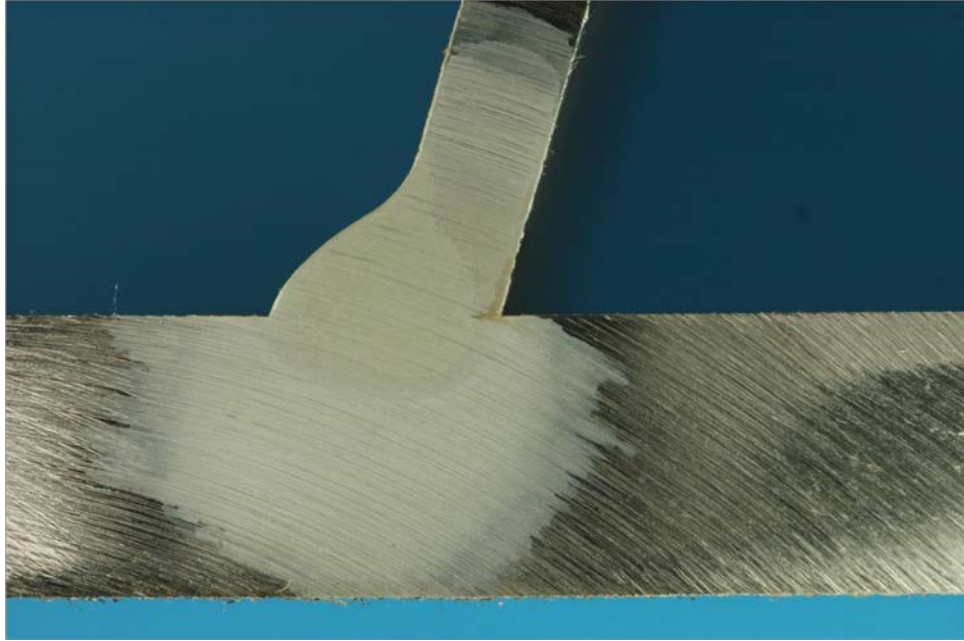
Figure 639. Macro-etched section A_120
