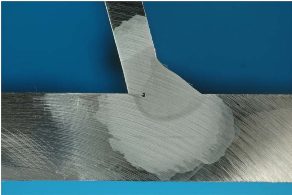
Figure 616. Macro-etched section R3_B_150
