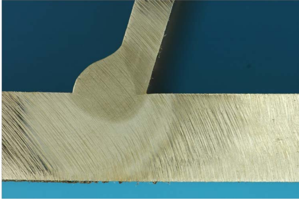
Figure 645. Macro-etched section A_156
