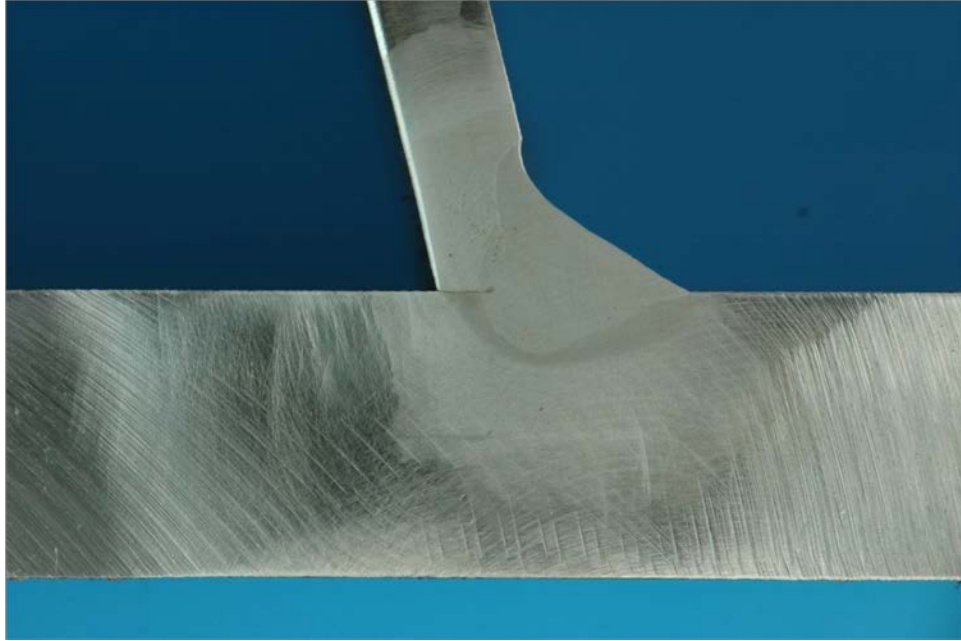
Figure 613. Macro-etched section R3_A_144
