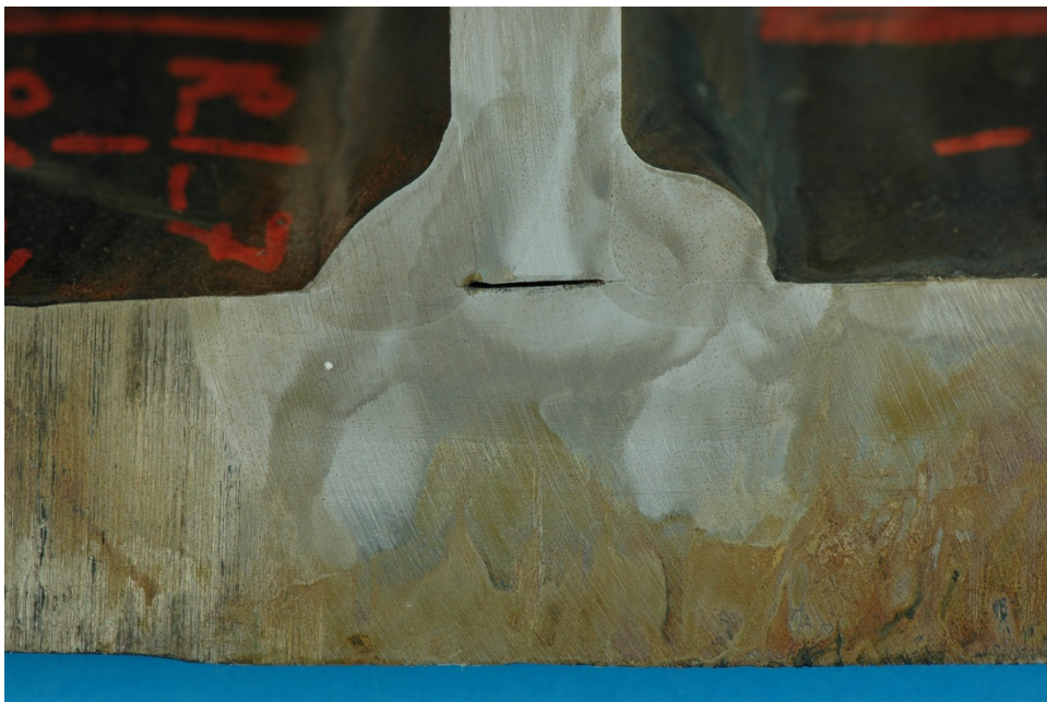
Figure 661. Macro-etched section R1_90_1
