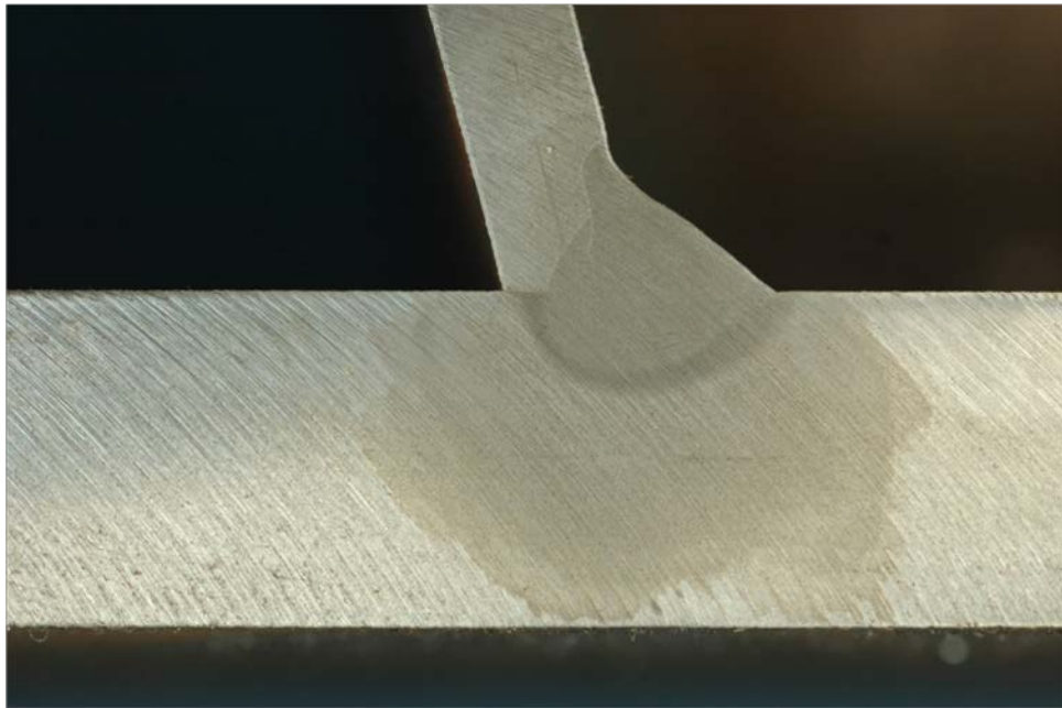
Figure 594. Macro-etched section R3_B_30
