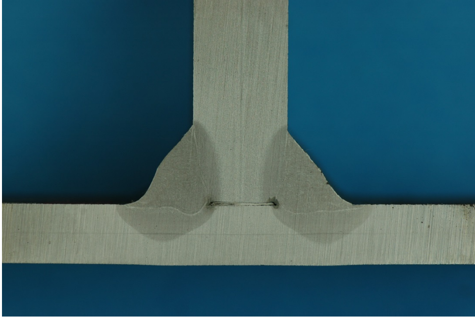
Figure 656. Macro-etched section R1_24_3
