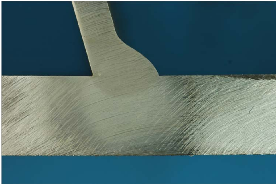
Figure 636. Macro-etched section B_96
