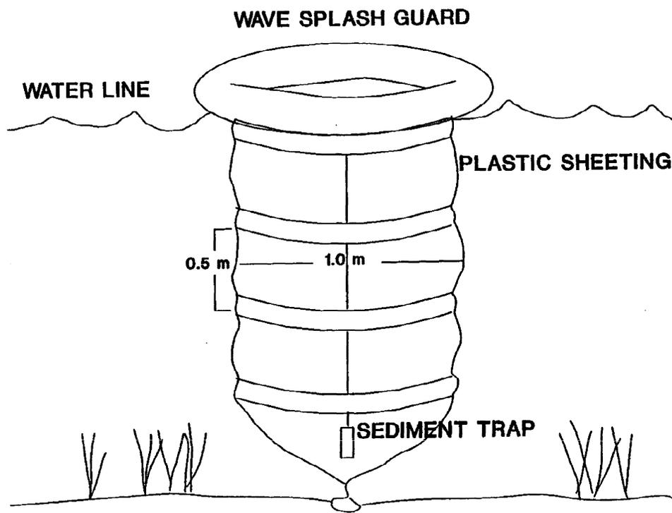
Figure 2. Water column enclosure with sediment trap for organic matter deposition measurements. See text for complete description of construction and use.
