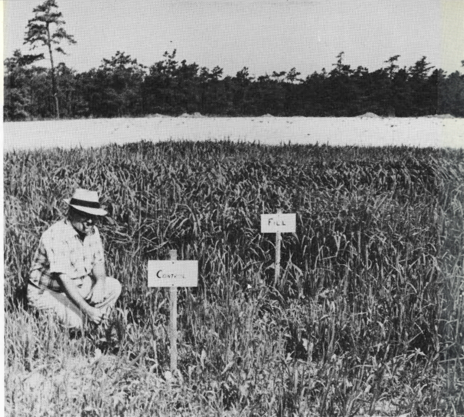
Since wildlife is a product of the land, soils research is an important program of the Bureau. Here Dr. Stephen Toth shows the results of adding river sediment to the sandy soils on the Colliers Mills Wildlife Management Area
