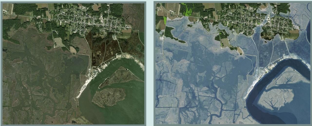
Figure 3.6 Delaware Bay Inundation, (L) Current and (R) 2-Foot Sea-Level Rise (NJCCRC).
