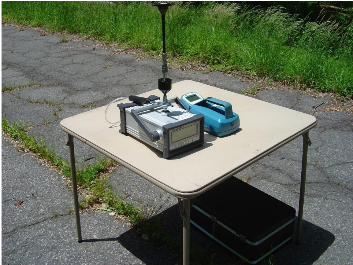
Figure 7: DataRAM and P-Trak instruments at ambient monitor station located 300 m from south west 0.1 mile turnaround loop.
