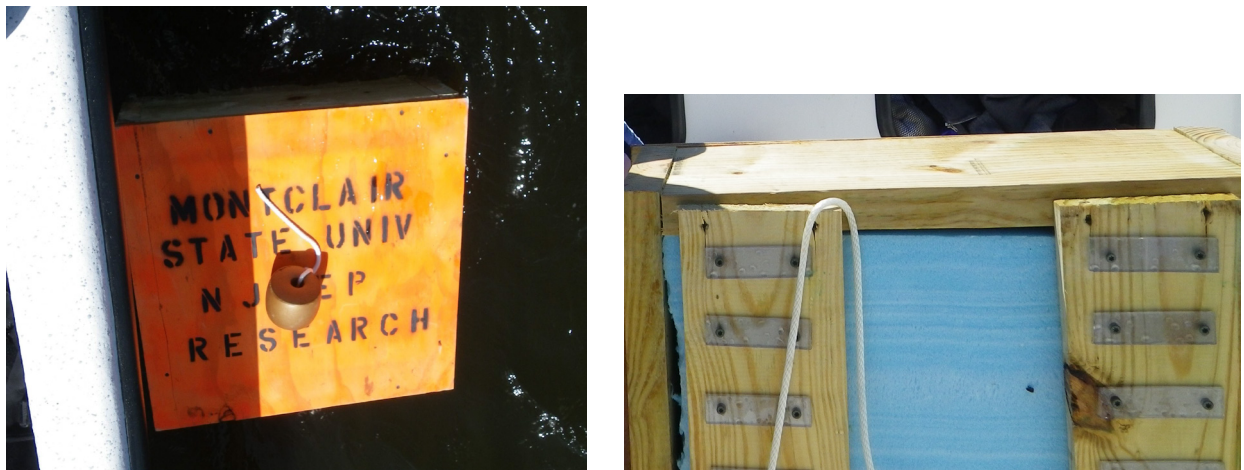
Image 3. Settlement Platform to assess larval settlement. A) Surface view floating on the water, B) Individual PVC settlement plates attached to the lower surface.
