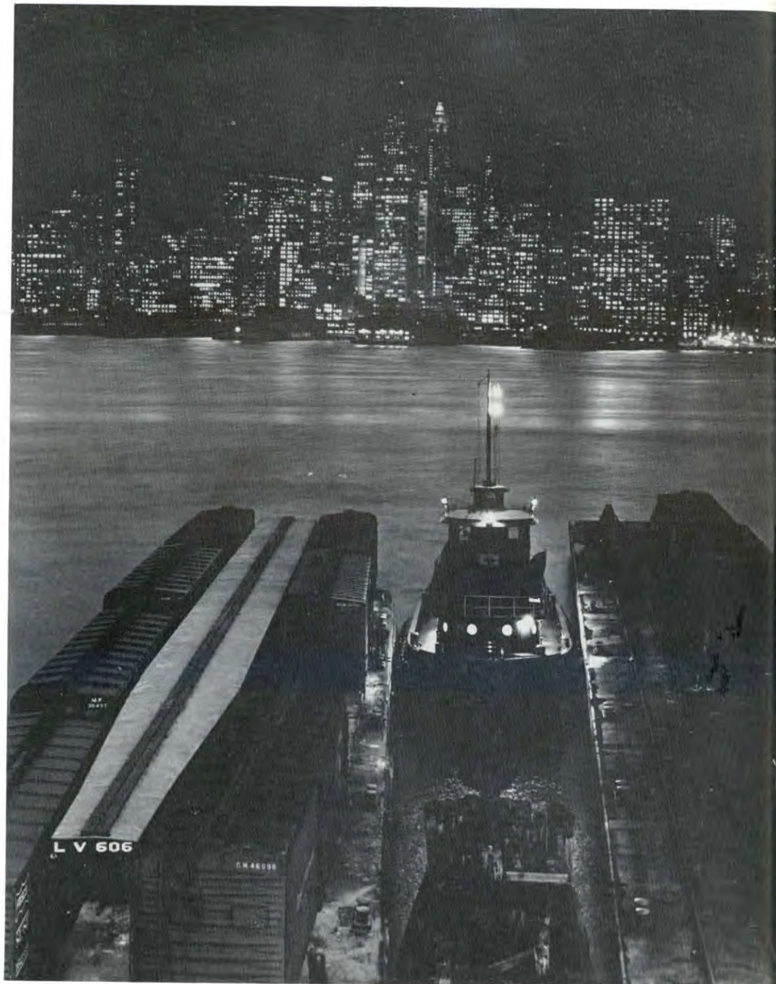
Night as well as day, activity goes on at the great New Jersey-New York Port. Here, a tugboat moves laden railroad carfloats into the Lehigh Valley Railroad yard on the New Jersey shore. Development of commerce in the Harbor is one of the Authority's chief responsibilities.
