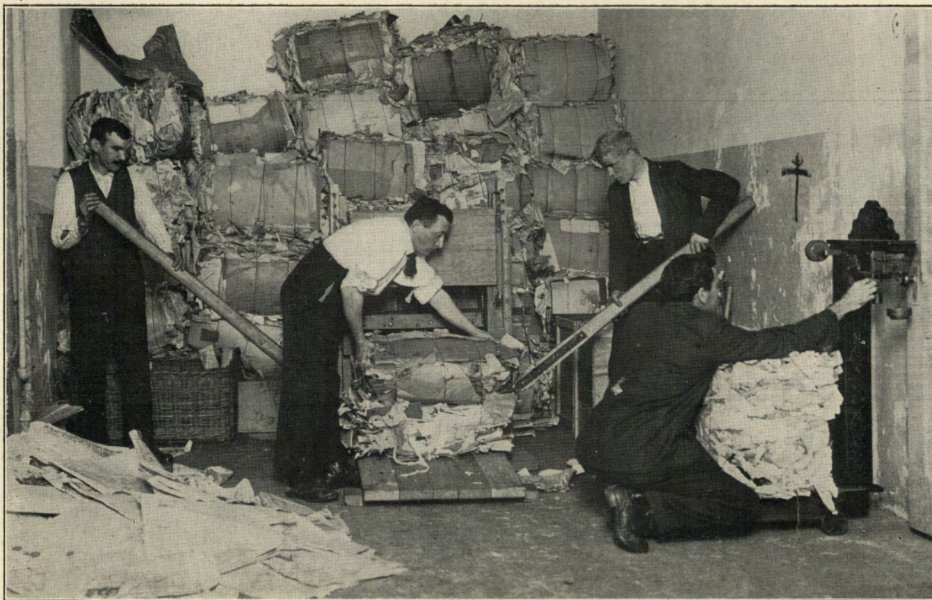
PATIENTS ENGAGED IN BALING WASTE PAPER IN PRESS CONSTRUCTED BY ONE OF THEIR NUMBER.
