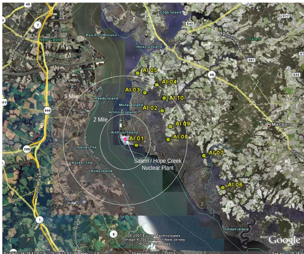
Figure 10 – CREST and Thermoluminescent Dosimeter Locations, Salem/Hope Creek
