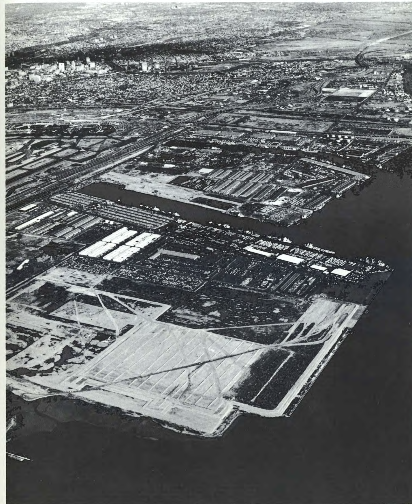
The location of the nearly completed Port Newark-Elizabeth Marine Terminal complex permitted reclamation of the large amount of supporting upland area required for container operations.
