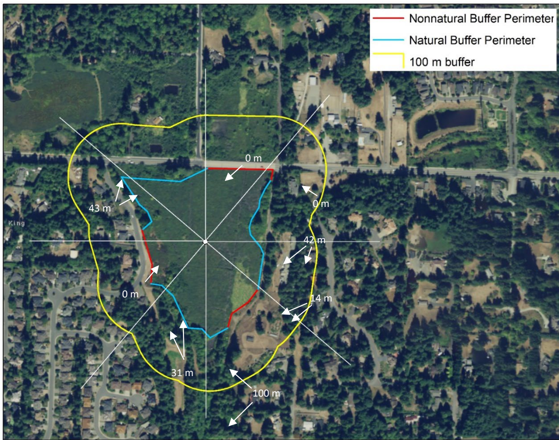
Figure 6. Buffer Width Calculation (point-based or simply polygons). The length of natural buffer is measured by calculating the distance between the edge of the AA and the 100 m buffer line along each of the eight white lines. Then an average is taken. In this example the calculation for average buffer length is (moving clockwise): (0+0+42+14+100+31+0+43)/8=28.75 m (Table 15). Consulting Table 17 this translates to a “C” rating.
