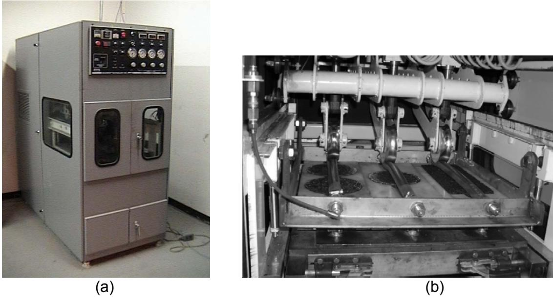
**Figure 27 – Asphalt Pavement Analyzer; a) Front of the APA, 2) Inside Testing Chamber of the APA**
