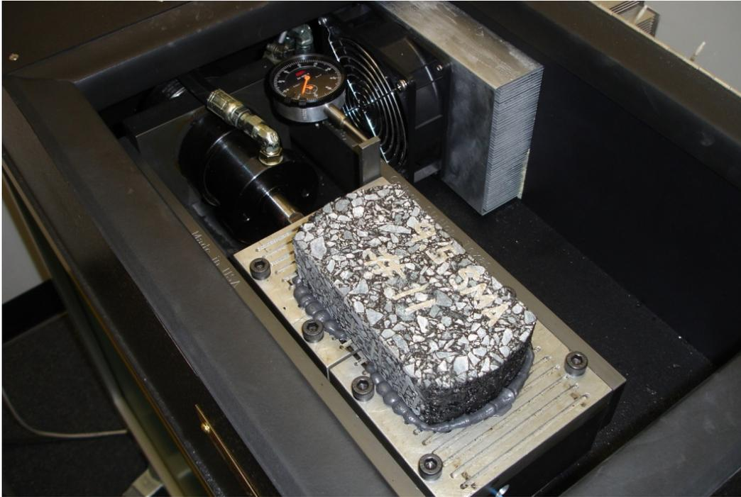
**Figure 26 - Picture of the Overlay Tester (Chamber Door Open)**
