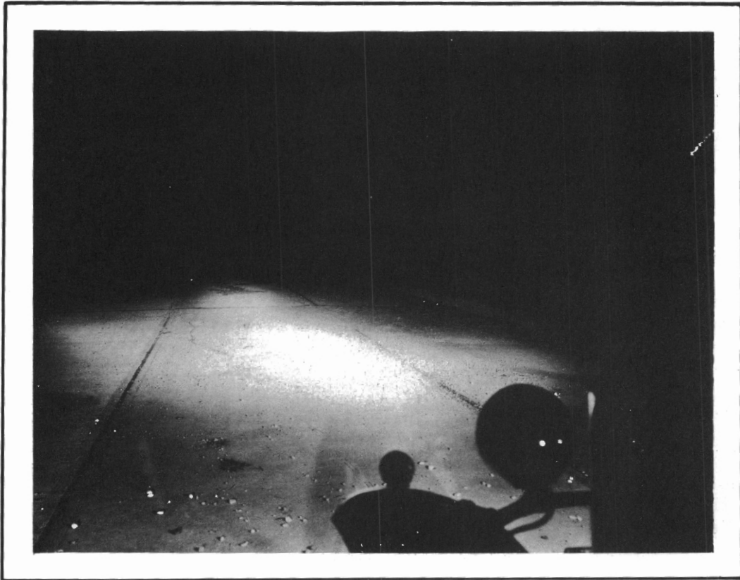
IN THE ABOVE PHOTOGRAPH THE MAN STANDING 70 FT. AHEAD OF THE CAR IS UNREVEALED BY THE AVERAGE HEADLIGHTS.
