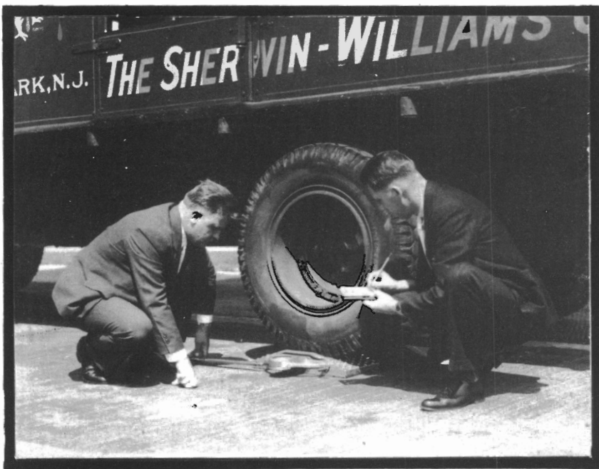
INSPECTORS WEIGHING TRUCK ON PORTABLE LOADOMETERS.
