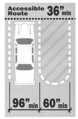
parking lot, and one in every eight accessible spaces, must be van-accessible with an access aisle at least 8 feet wide. The parking spaces and access aisles must be painted in a color (most often blue) contrasting with other spaces. Signage with the International Symbol of Accessibility and the Penalty Sign MUST be provided at each handicapped parking space and must be permanently installed 5 to 7 feet above the ground.
