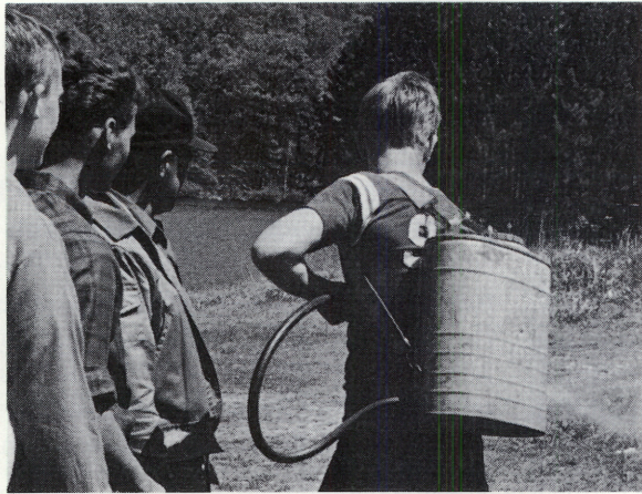
The forest fire warden demonstrates fire fighting techniques and equipment. The student is practicing how to use an Indian back tank and pump
