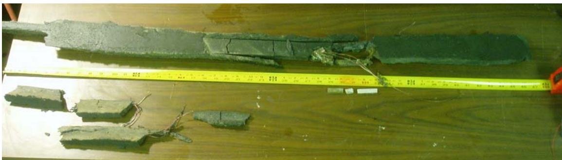
Recovered sensor assembly from Rt. 287 field installation
