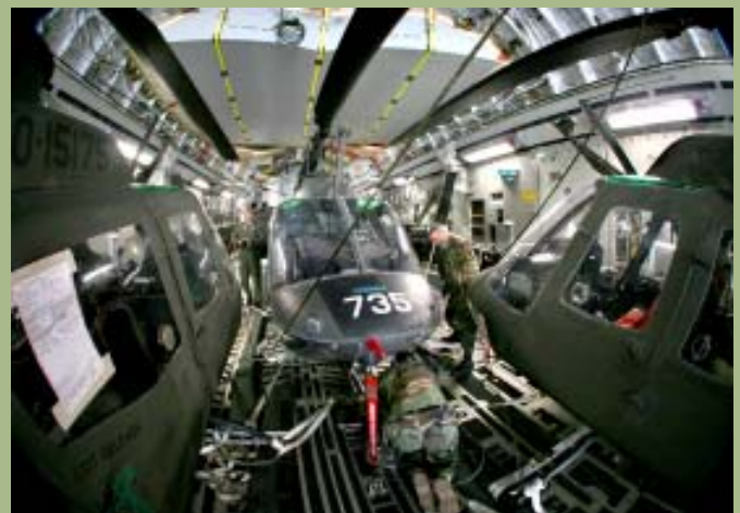
Tight quarters for the five OH-58 Kiowas on board the C-17.
