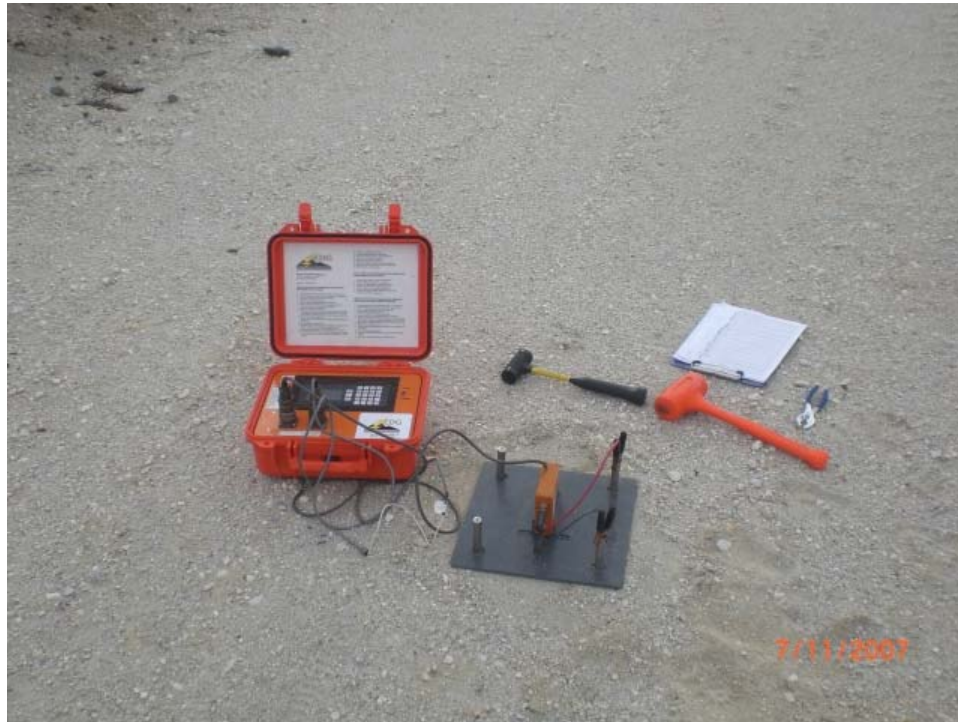
Figure 4 - Electrical Density Gauge (EDG) Setup
