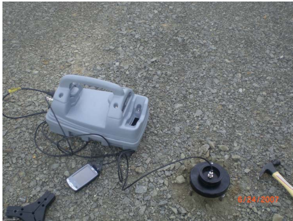
Figure 3 - Moisture Density Indicator-MDI 2000 (TDR) Setup
