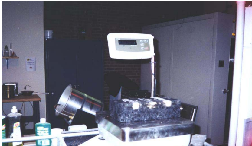
Figure 21 Weighing of samples to determine saturated surface dry (SSD) weight.
