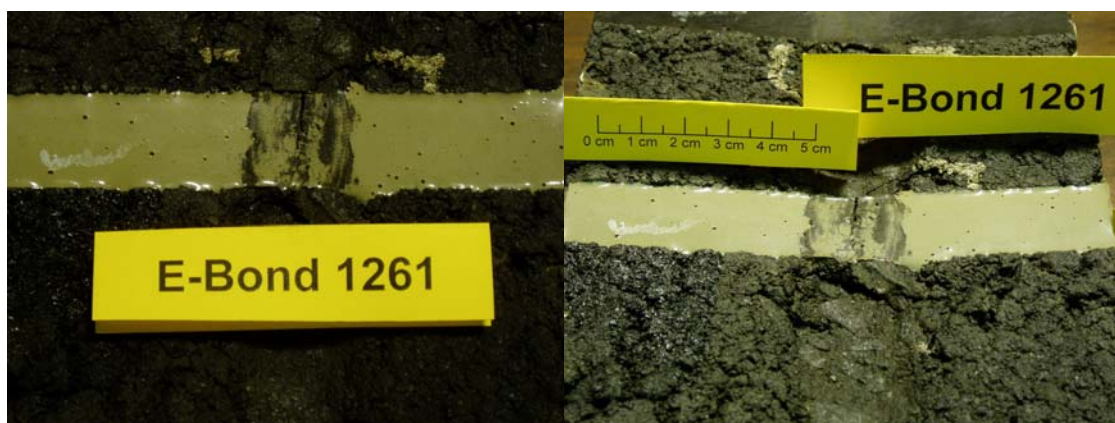
Figure 14 Photograph of APA Test rutting results of E-Bond 1261.
