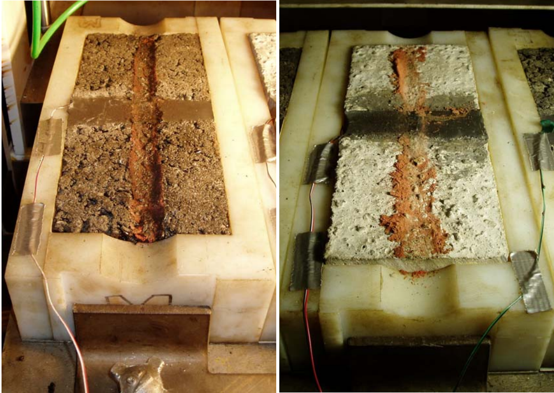
Figure 33 Photograph of rutting effects on the asphalt pavement (left) and concrete pavement (right) samples.
