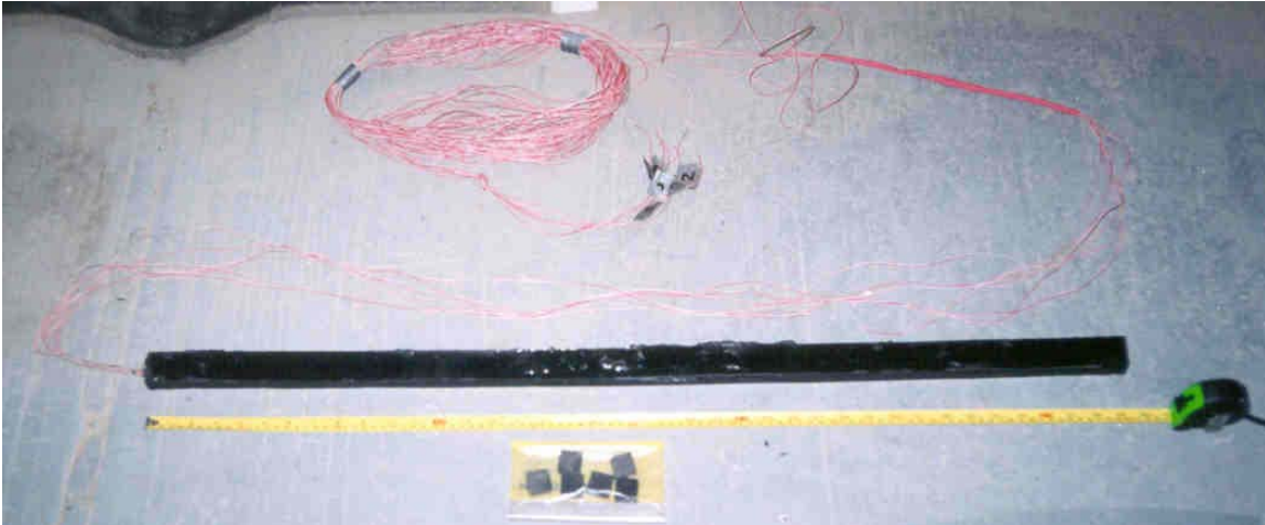
Figure 56 Photograph of ceramic-polymer composite sensor assembly and chairs laid-out in the laboratory.
