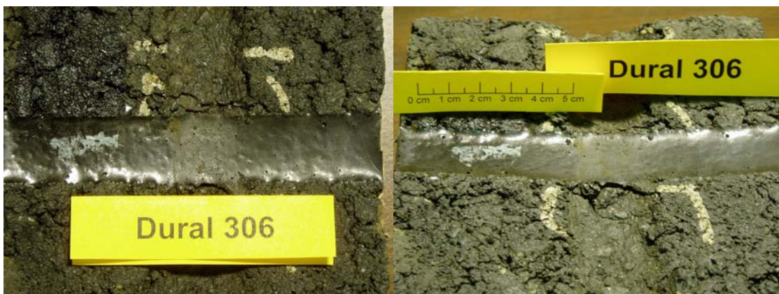
Figure 15 Photograph of APA Test rutting results of Dural 306.
