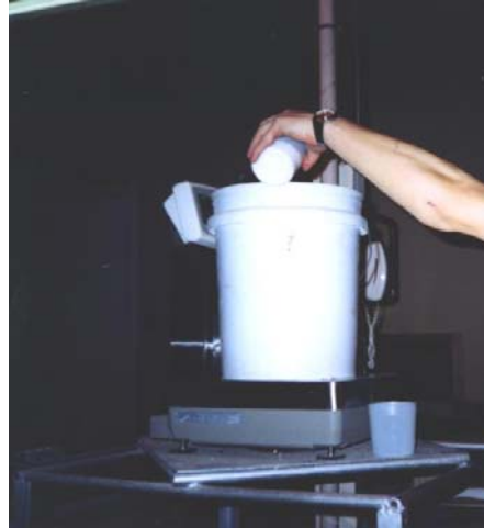
Figure 20 Addition of salt to form brine solution to ensure test would be performed under worst case environmental effects.
