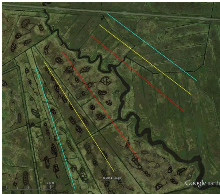
Figure 4. Established line transects on the OMWM and control sections of the AT & T site. On each side, transect 1 is red, transect 2 is yellow, and transect 3 is blue (oriented by proximity to the large tidal channel).
