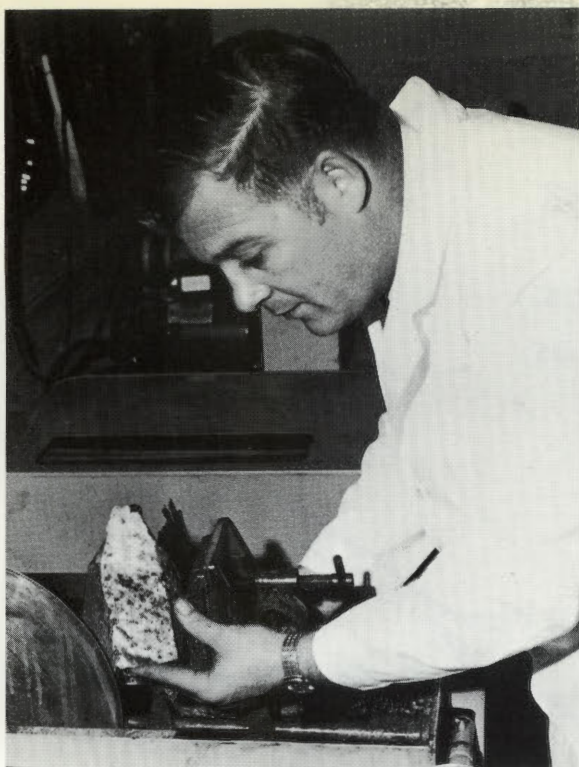
Dr. E. Everett MacNamara, Research Assistant Professor in Lehigh University's Center for Marine and Environmental Studies, prepares to slab-cut a rock specimen from Antarctica in order to make a thin section for mineralogical investigation
