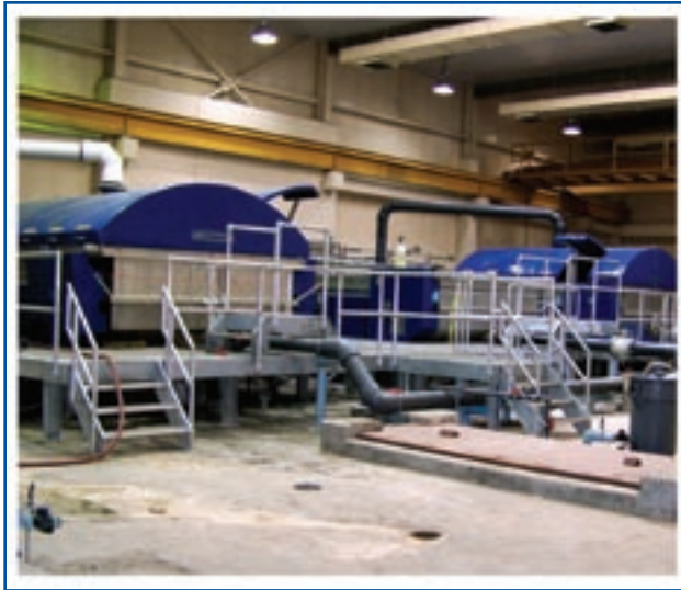
Camden County Municipal Utilities Authority - sludge dewatering equipment.
