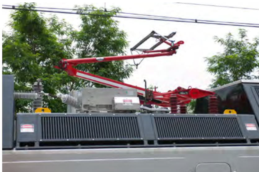
New dual-mode locomotives transition between diesel fuel and electricity, providing greater operating flexibility.
