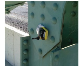
Top: Illustration of sensor placements. Bottom: Sensor on steel truss member.
