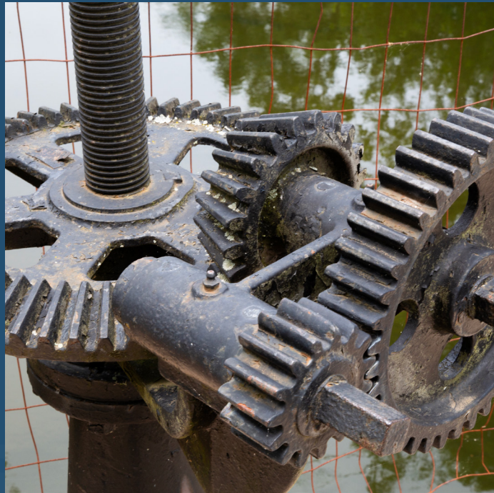
Delaware and Raritan Canal lock control gears in Bulls Island Recreation Area.
