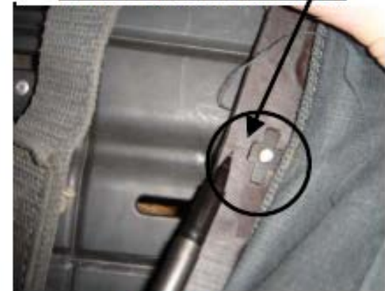
Crack At Lumbar Support Caused Separation Failure
