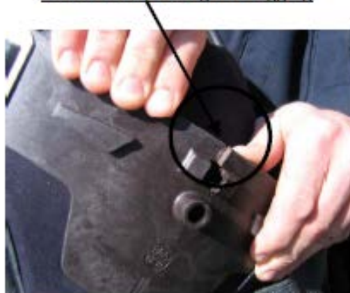
Crack From Pulling & Dragging
