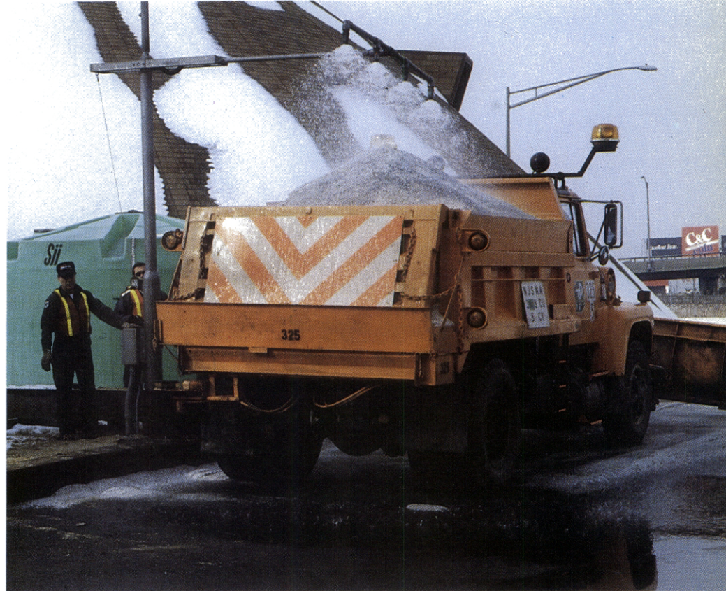
SPRAYING SOLUTION of calcium chloride on rock salt proved successful in reducing cost and increasing efficiency of snow and ice removal operations.
