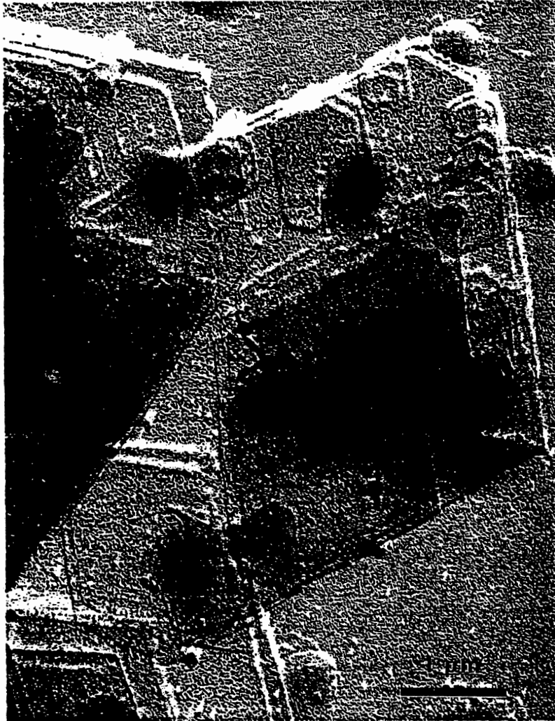
FIGURE Bright field image of shadowed multilayered solution-grown polyethylene crystals. A rather heavy shadowing deposit has been used for clarity.
