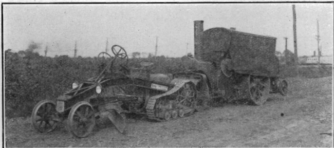
COUNTY SCRAPER AND ROLLER USED FOR ROAD REPAIR
