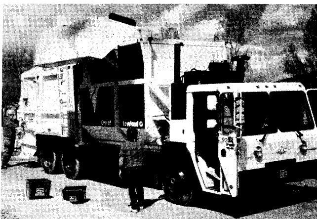
Loveland's semi-automated dual-collection vehicle. Crews put recyclables into the split side-loading compartment and trash into the rear-loading packer compartment.
