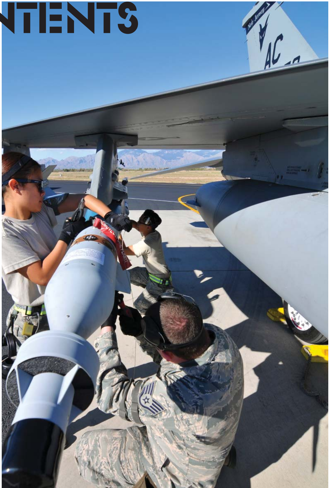
Above: Weapons loaders, left to right, Senior Airmen Jerilyn Co and Andy Nguyen and Staff Sgt. Chris Miller with the 177th Fighter Wing, load a GBU-12 laser guided bomb on an F-16C Fighting Falcon during Operation Snowbird at Davis-Monthan Air Force Base, Ariz., March 3, 2014. (U.S. Air National Guard photo by Master Sgt. Andrew J. Moseley/Released)
