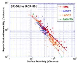
3. The addition of SCMs to the mixture proportions favorably reduces the RCP measurements and
