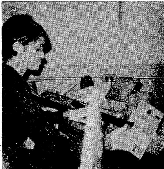
Film Cutter positioning film in machine to cut strip into multiple units.
