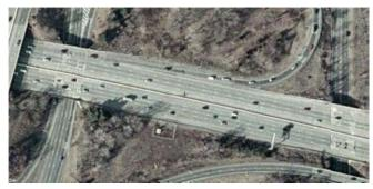
specifically among the initial tasks a limited field measurements was also conducted. These were two bridges on I-80E over I-287N and the Smith Road. The former is a steel bridge while the other is a reinforced concrete bridge. Both bridges have similar structural stiffness and satisfy AASHTO deflection
