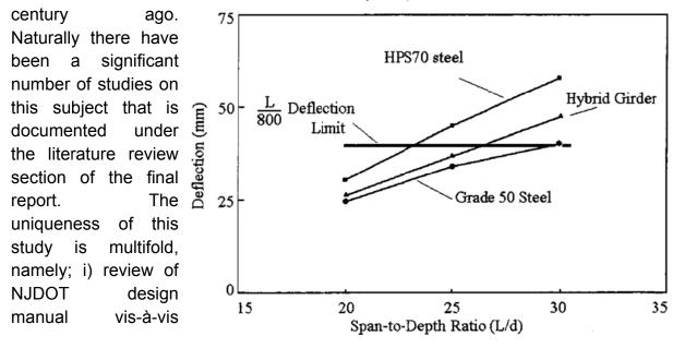
serviceability requirements as despite the fact that AASHTO has made these requirements optional, they are used by NJDOT, ii) Appropriateness of the listed spanto-depth ratios and to establish ratio limitations that address the use of higher structural steel grades, and iii) most importantly propose the "next generation" serviceability requirements that ensures human safety and structural performance while facilitating applications of high performance materials.
