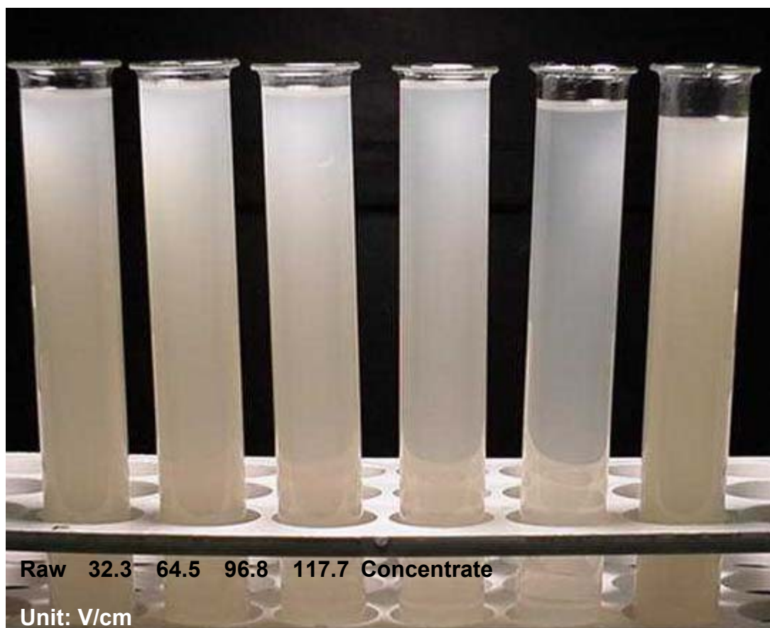
Figure 10. Visual comparison of water samples treated at various levels of electrostatic field (well #5S, high flow purging sample)
