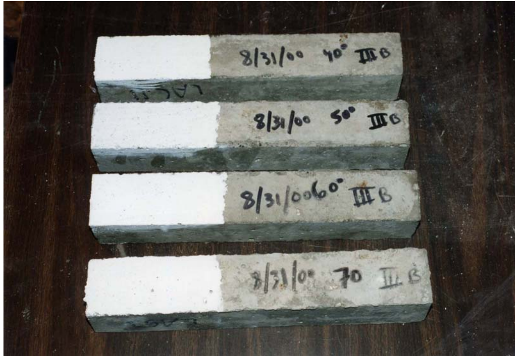
Figure 2.1(a) Concrete Prisms Coated with Geopolymer and Exposed to Running Water
