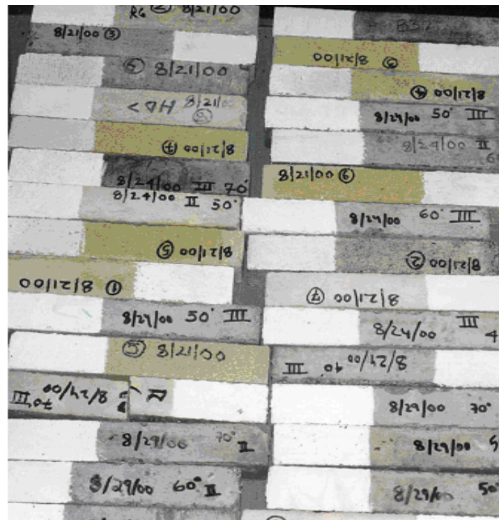
Figure 2.1(b) Concrete Prisms Coated with Geopolymer and Exposed to Running Water
