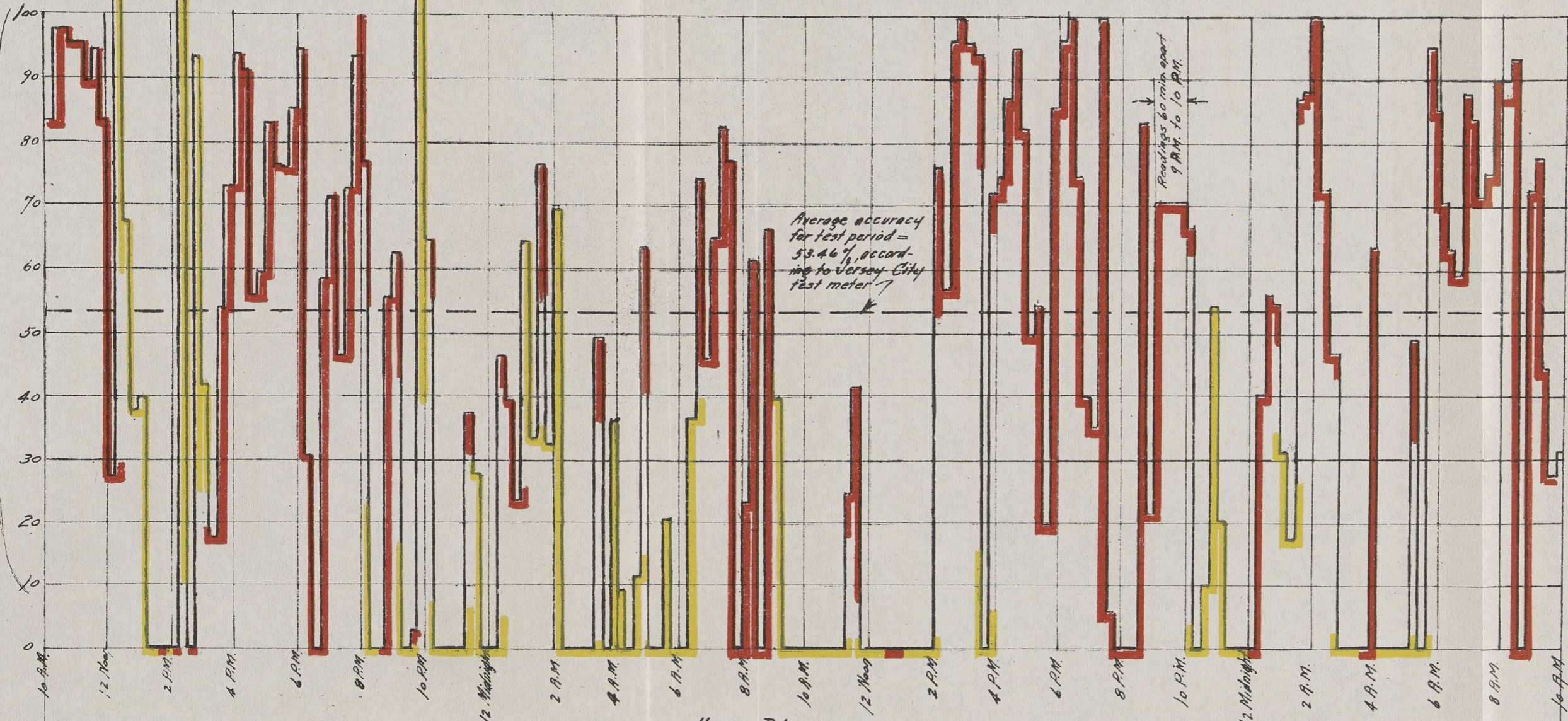
Upper Diagram Accuracy percentages of Hershey meter during test by Jersey City. Scales { Horizontal: 1 inch = 2 hours Vertical: 1 inch = 10 per cent.
