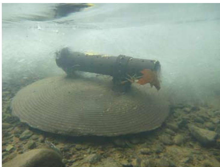
This is one of the six continuous conductivity monitors being used by DRBC staff to collect important baseline information in the upper basin.
