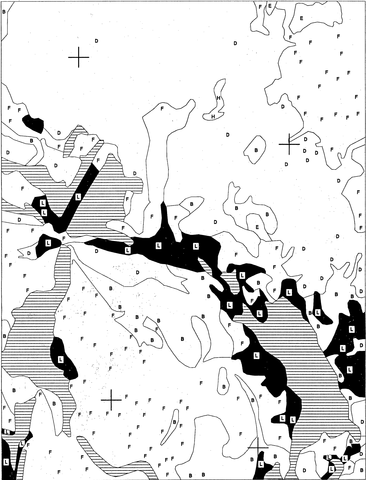
Figure 20. Step 3b: Soil group overlay showing soil-group symbols, boundaries and shaded hydric soils.
