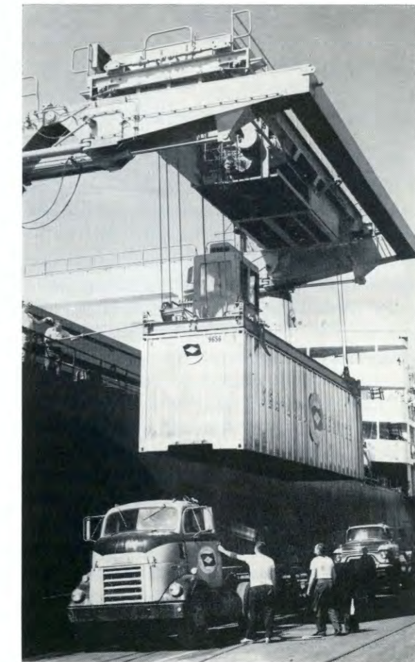
Port Newark's container ship service by Pan-Atlantic Steamship Corporation has two vessels capable of lifting trailer-like container bodies from trucks' chassis and stowing them aboard.
