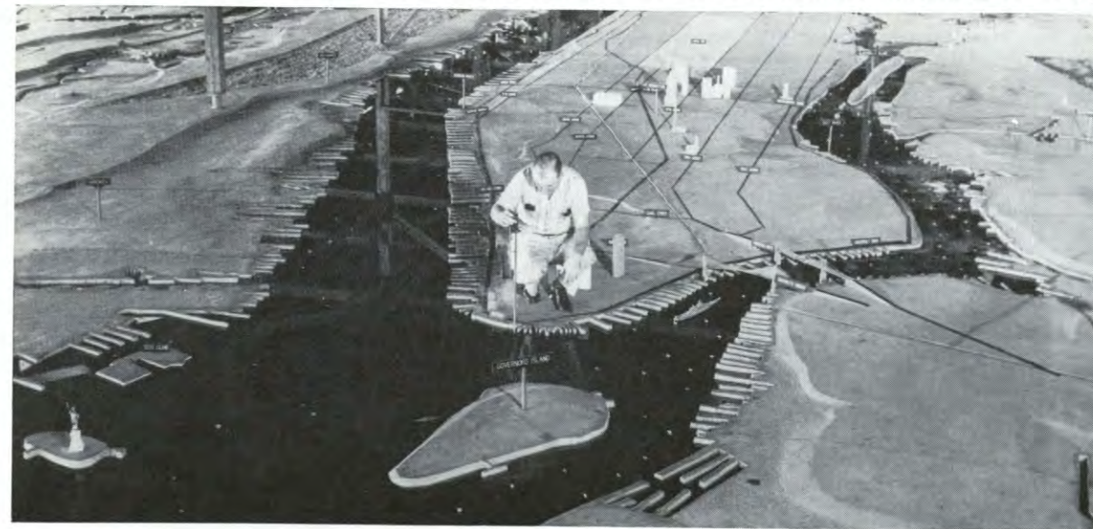
At Vicksburg, Mississippi, the United States Army Corps of Engineers' model of the entire New York-New Jersey Port area duplicates water action in the "harbor" and aids in studying many problems, including siltation. Specialist in center kneels on the "Battery."
