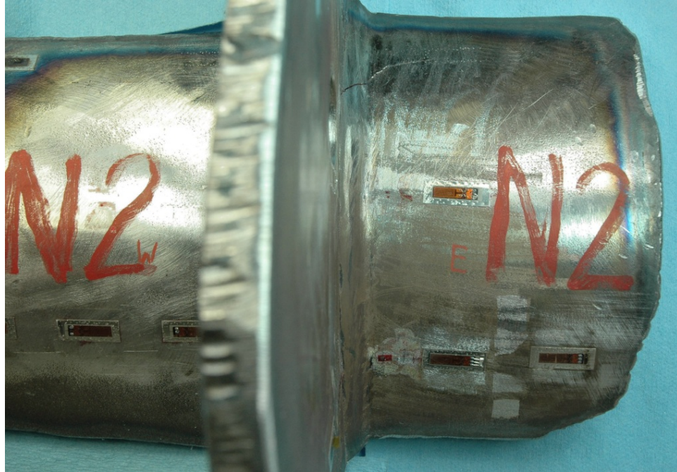
Figure 211. Portion of rib and floor beam containing the north side crack cut out of the mock-up specimen MU2
