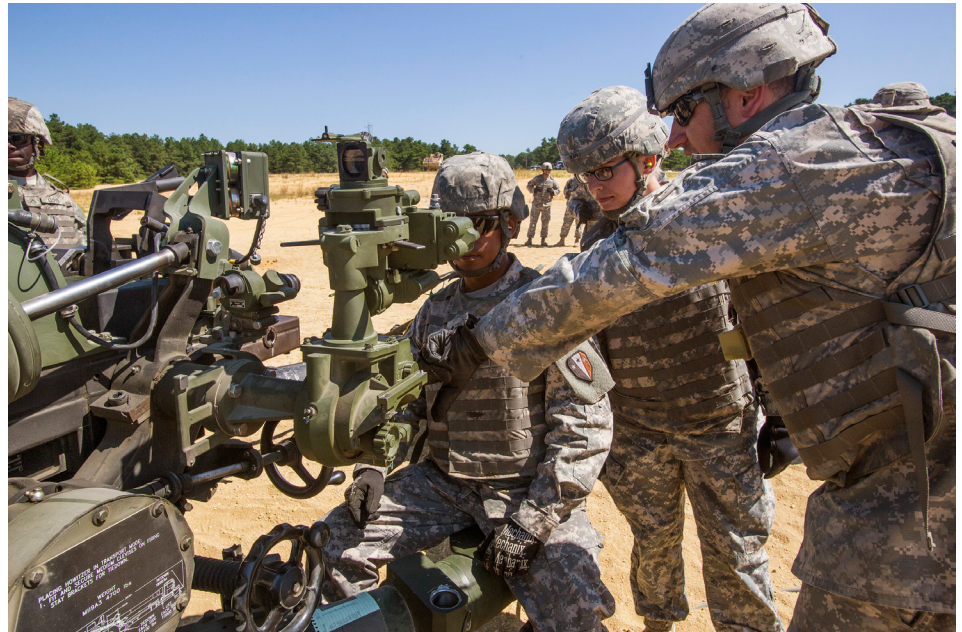
Staff Sgt. Bryan Young, right, and Sgt. Santiago Sanchez, left, show 2nd Lt. Jennifer Wain, all with the 3-112th Field Artillery, the sighting system on the all-digital M119A3 105 mm lightweight howitzer during a live fire exercise at Joint Base McGuire-Dix-Lakehurst, N.J., Aug. 26, 2015. The upgraded M119A3 is equipped with a digital fire control system that includes an inertial navigation unit, guided-precision system technology and other features that will give the weapon the ability to determine its precise geographical location on its own. (U.S. Air National Guard photo by Master Sgt. Mark C. Olsen/Released)
