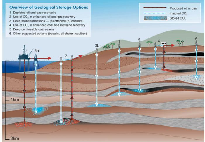
Figure 1. Types of CO<sub>2</sub> Geological Storage Options. In New Jersey, deep saline formations, both offshore (3a) and onshore (3b) offer the best potential for geological carbon sequestration. *Figure from <u>Intergovernmental Panel on Climate Change</u>*
