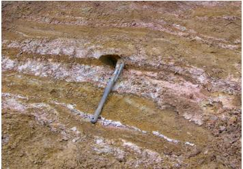
Figure 1. Clay beds and interbedded sand in the Cohansey Formation, exposed in a cut near Forked River Mountain in the Brookville quadrangle. Clay beds are pink to white, sand beds are browbn to yellowish-brown.
