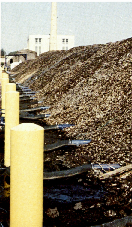
Long rows of wood chips-sludge mixture are aerated to encourage the composting process. This part of the process takes about 21 days.
