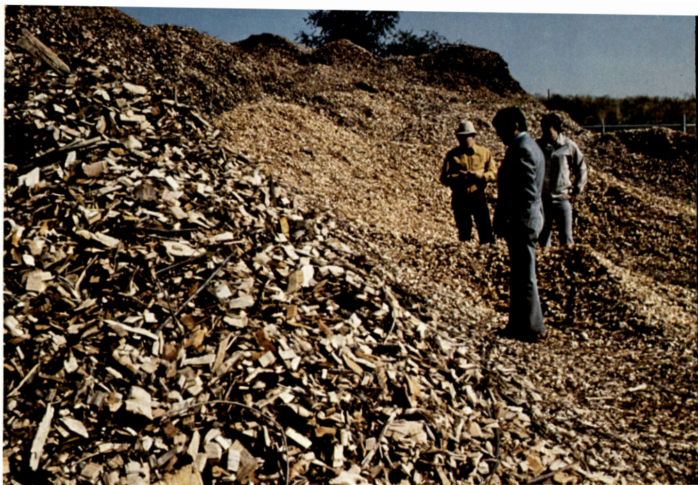
Wood chips, to be used as bulking agent material for the composting process are purchased and stored on site. To this point approximately 13,000 cubic yards of chips have been delivered to the Camden facility.
